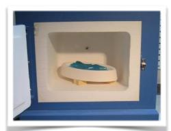
Fire the molds according to the Component Casting Schedule. The low temperatures of this schedule will preserve the designs' delicate edge detail and keep the glass from "balling up" due to sur-face tension.
