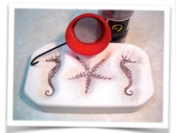
Remove any existing kiln wash using a stiff, nylon brush. Spray the mold with ZYP as described above, but using a two to threesecond blast since the mold is smaller. Just as before, spray the mold twice if this is the **fi** rst time the mold has been treated with boron nitride.
