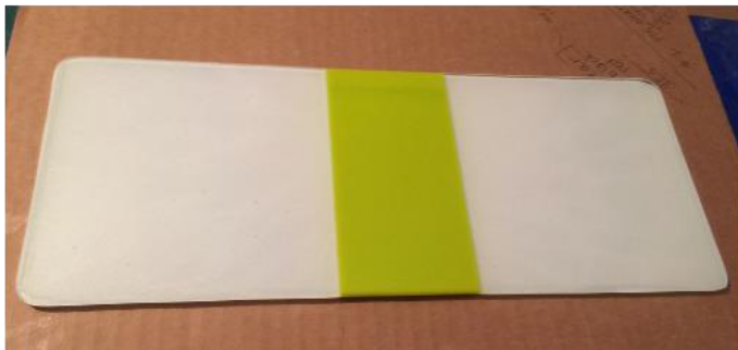
The bottom of the piece after the project is fused and removed from mold.
