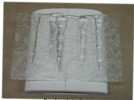
Panel ready to slump
