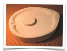
This plug is used to make a hole in the cast leaf. Note: If 1/8" fi ber paper is not available, use a combination of other thickness to get the same results.
