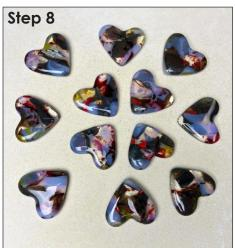
Once each cavity is full, transfer the mold to a level shelf in the kiln and fire using the suggested schedule in **Table 1** or your own preferred Full Fuse. If using fill weights, each heart should have around 31 grams of glass.
