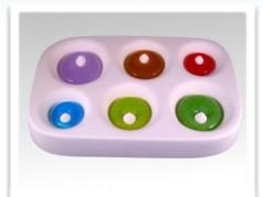
Of course, the perfect firing schedule for your kiln will depend on ambient temperature, glass color, kiln load, kiln age and whether the kiln has top or side elements. If you notice that that the corners of your Offset Square Pendant castings are significantly rounder than those of the mold, reduce the target temperature in subsequent firings.
