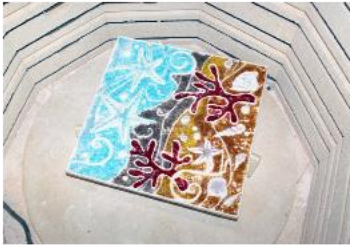
Image 6: The fully-filled texture mold on kiln posts in the kiln before being backed with sheet glass
