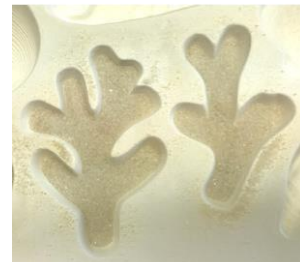
Add F2 Khaki until smaller cavity holds 19 grams total and the larger holds 25 grams total.
