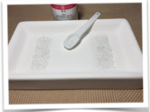
The feet of the Slab Server are filled with coarse frit so the sheet glass melts evenly
