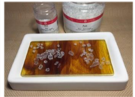
Coarse frit is placed on the top surface to displace the pattern in the sheet glass
