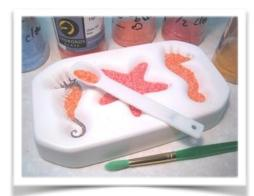
To make our samples, we used fine mesh frit. Further, we mixed our frit colors with equal amounts of fine clear frit. The results were more subtle, less saturated castings.
