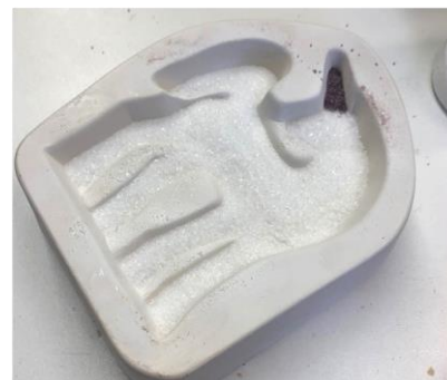
Back everything but the horn with F2 White until the mold is uniformly 1/4" full of frit (about 30 grams).
