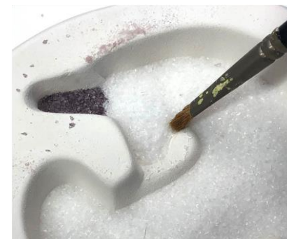
Gently sweep the frit back from the mold walls and fire to a Tack Fire using the suggested schedule in Table 1 or your own favorite Tack Fire.
