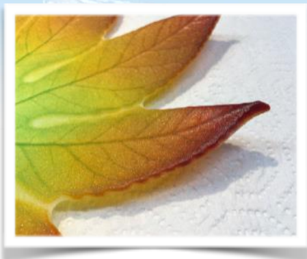
Castings are only about 2mm thick
