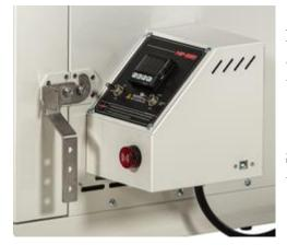
**Programmable Alarm:** Each unit comes standard with an integrated alarm that can be set to alert the user when a desired point or temperature is reached in the program.
